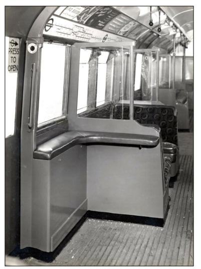
One trailer oddity on the Northern Line was trailer 012339 (*Left*), which was given additional stand-back areas around the double doors, but at the loss of eight seats. Again, this offered a 1 in 100 chance of it being seen 'on the road' at peak times.
