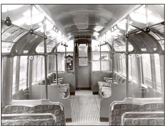
**Above:** 1938 Tube Stock UNDM 30016, converted from a nine-car NDM in Golders Green Depot (*Left*). Interior of a 1949 Tube Stock UNDM (*Right*). The shunting control panel can be seen in the distance to the left of the communicating door.
